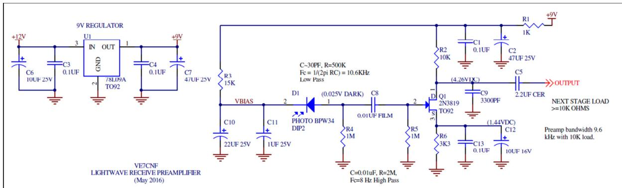
Link to PDF version of schematic: [VE7CNF\\_LW\\_RxPreamp.pdf](#)
